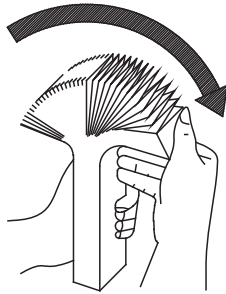
Fig. 5.1-5 Loosening the Chart Paper
